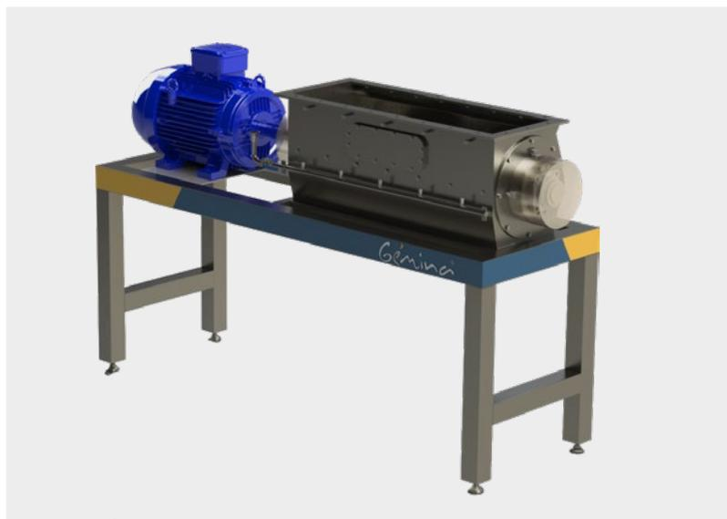
Then, the product is placed over a sieve fitted in the surrounding movement area of the hammer blades. Here, a second stage of breaking is produced by shearing and the product goes through the sieve holes and leaves the main hopper.
