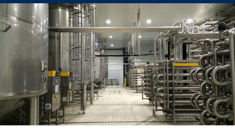
**66** Six processing lines compounded by pasteurizer and aseptic tank. All the equipments are combined thanks to a completely automatic mixing room which has included recipes management and recipes control.
