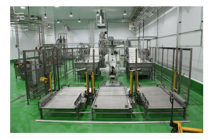
New development for the production of melons and watermelons: extraction of the pulp without mashing and mixing the outer rind, which produces an exquisite quality pure melon or watermelon cream ready to be refined and clean of seeds before the heat treatment previous to the aseptic packaging.
