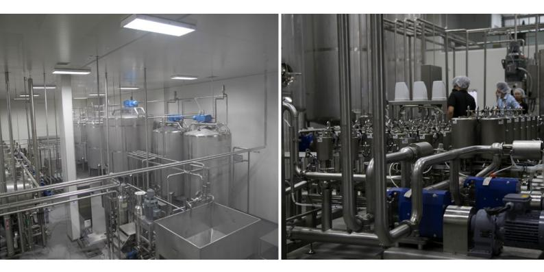
Automatic raw material room with preparation and recipe record for dosage of different ingredients such as chili, sugar, pieces of vegetables, garlic sauce... and combining a kitchen of 7 heated tanks with mixing for recipes preparation.
