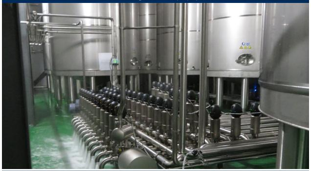
System which combines multitrack equipment for combining different stages of the process according to the specific procedure in each product.
