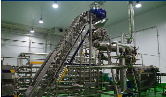
Line including thermophysics peeler for tomato peeling and its following grinding for packaging in tubs.
