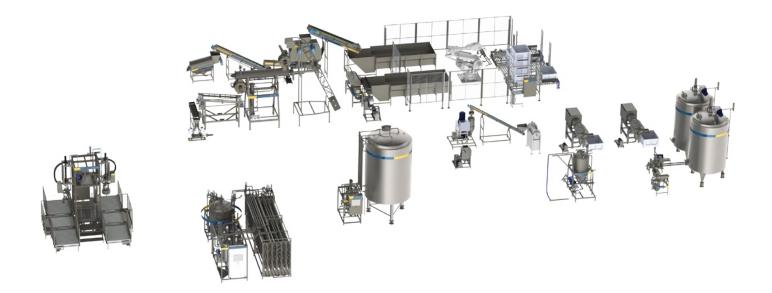
Reception of raw material: A robot feeds two different processing lines with pallets of fruits and vegetables weighing 400 kg each one. One line processes all kind of fruits and vegetables, and the other line is conceived for processing melons and watermelons.
